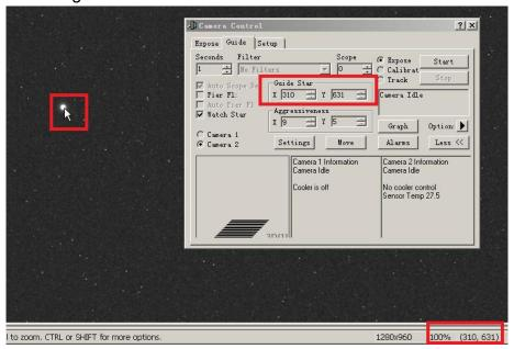
8. Click "Setting" to make sure that Autoguider Output is "Guider Relays". Then MaxIm\_DL will use the ST4 port on the camera to guide. Or choose "ASCOM" driver to connect "ASI Camera ST4 telescope driver" if you connect camera through WDM driver.
