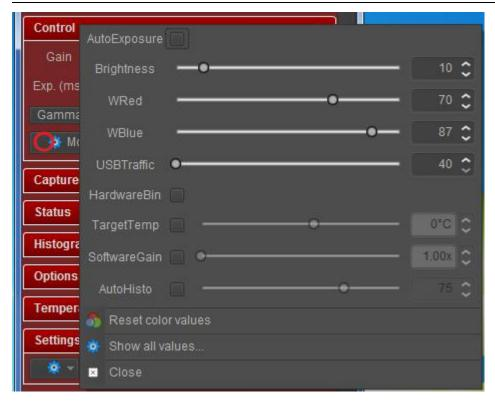
For cooled camera, enable the check box in control "TargetTemp" to turn on auto cooling, sensor temperature and cooler power is shown on title bar of image display panel.
