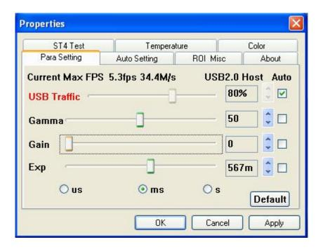
This is very important to adjust "USB Traffic" to a suitable value to match your PC, this depends on the USB controller. And you may need to adjust it lower if there is other device to share USB bandwidth with your camera.
