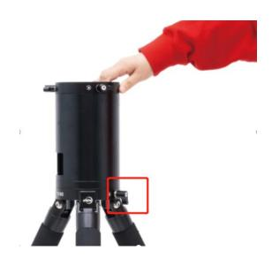
Insert the multi-function support bar as shown in figure below (see figure 1), rotate the knob on the multi-function support bar clockwise and tighten it, then fit the tripod spreader and rotate its knob clockwise to lock it in place.
