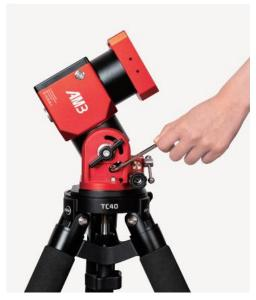
At this point, the mount is in the second gear position. In this state, the mount can adjust the altitude angle within a range of 30° to 90°. After completing the adjustment, tighten the altitude gear tension knobs.
