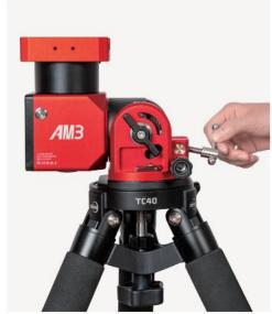
Loosen both hex screws on the sides completely by turning counter clockwise with a hex wrench.
