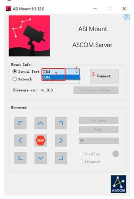
\* Note: The port number to select can be found in Computer Management, as shown below. Alternatively, you can try each serial port provided in the ASI Mount ASCOM interface one by one.
