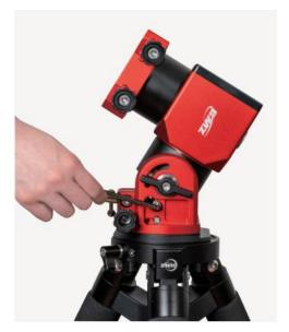
Move the mount head to slide and adjust the "altitude gear fine adjustment knob". Slide the hex screw to the bottom end of the sliding rail in the hole, with the scale screw indicating 90°. At the same time, re-tighten the hex screws on both sides. (Note: After adjusting the altitude gear, be sure to tighten the gear screws firmly, otherwise the equipment may become loosen and the gear adjustment function can be easily damaged.)
