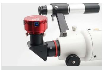
3. Take off the eyepiece on the telescope and install the camera.
