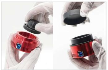
1. Screw off the fisheye lens and the black adapter of the camera (if any), or take off the dustproof cover
