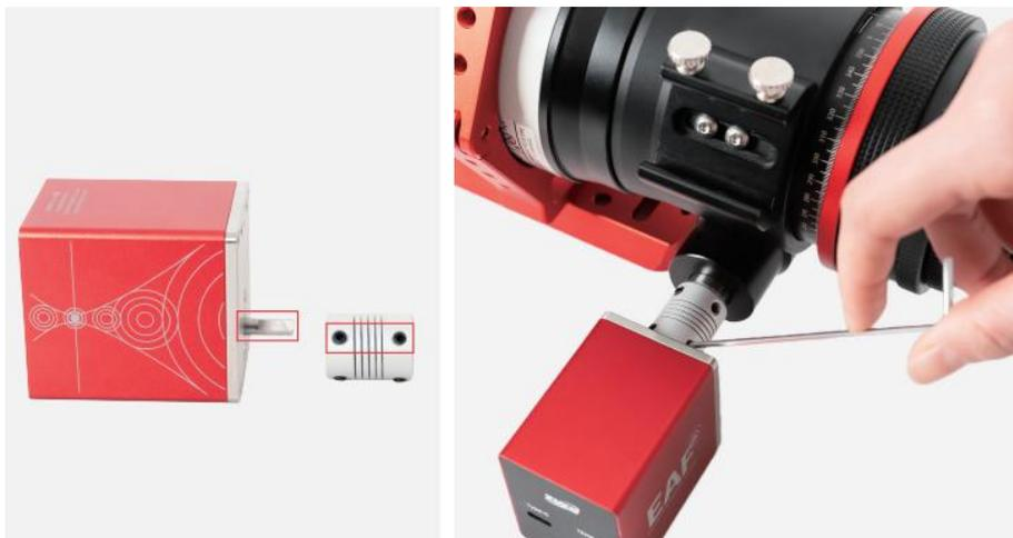
Secure the EAF body to the bracket and the bracket to the matching mounting holes in the focuser assembly using the supplied M4 screws. Ensure that the bracket is flush with the EAF mounting surface without any gaps, and that it is parallel to the focuser body surface.
