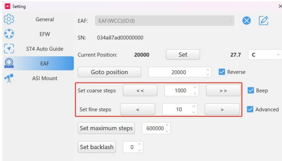
**Move Outward:** Click the coarse button to move the EAF out by 1000 steps.
