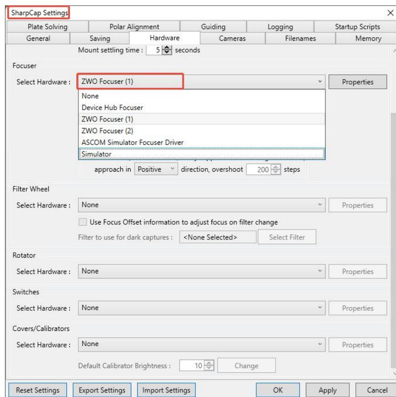
Click the “Properties” button to open the “EAF Setup” window automatically. Here, you can configure basic parameters and perform manual focusing operations.
