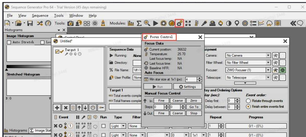
Refer to the "EAF Parameter Settings" section to set the zero position, upper limit, and backlash. Additionally, set the step size according to your preference.
