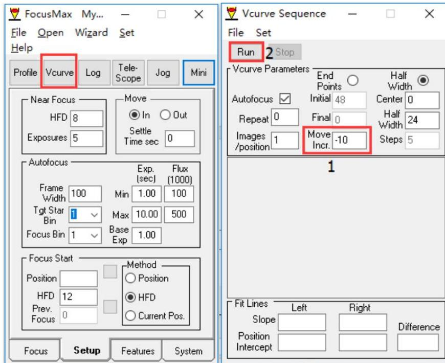
After the V curve is drawn the focuser will be driven to the optimal focus position.
