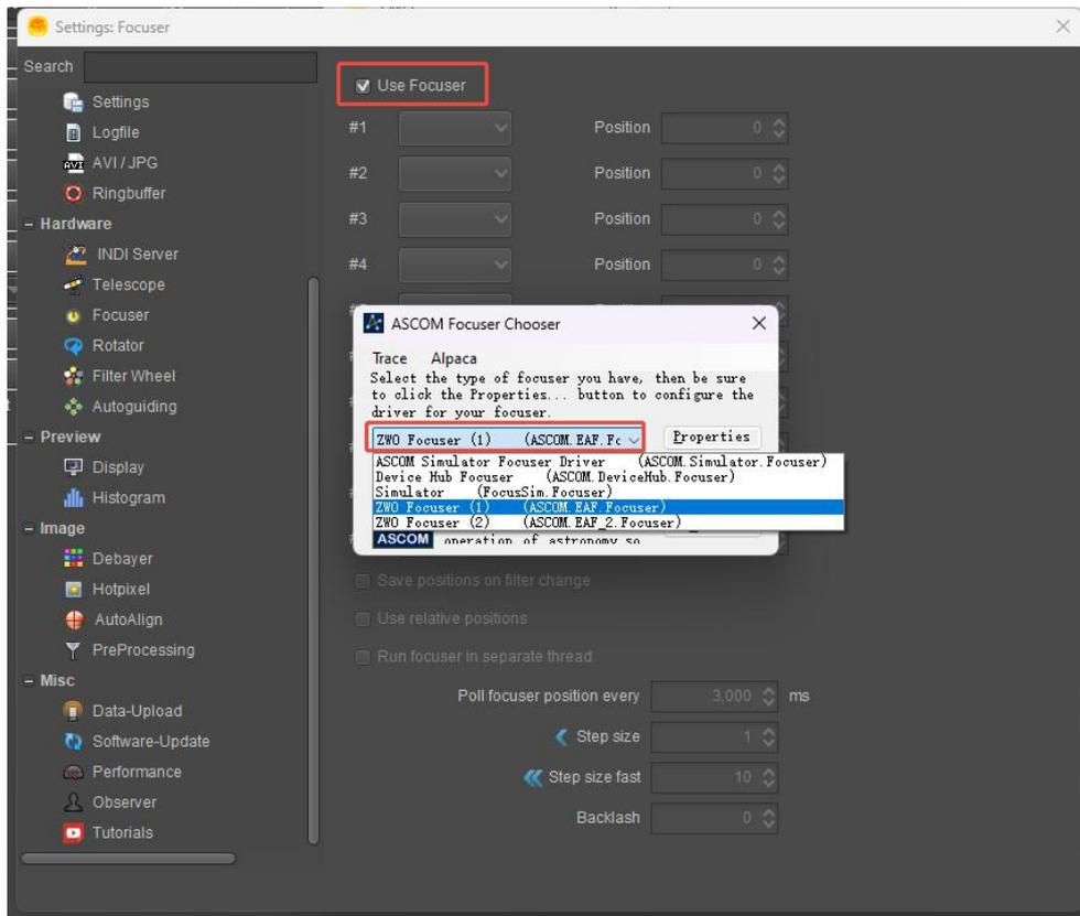
Click “Properties” to open the “ZWO EAF Setup” page, where you can configure the EAF parameters and perform manual focusing operations.
