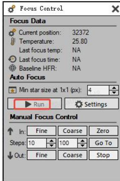
SGP will automatically capture images and adjust the focus while plotting a V-curve. Once the focusing curve is completed, SGP will drive the EAF to the calculated optimal focus position. Autofocus is then complete.
