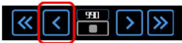
**Measure Backlash:** Continue clicking the inward fine adjustment button one step at a time while observing the focuser knob. When the focuser knob starts to rotate, it indicates the backlash has been taken up. The number of clicks before the focuser knob rotates multiplied by 10 is the backlash step count.
