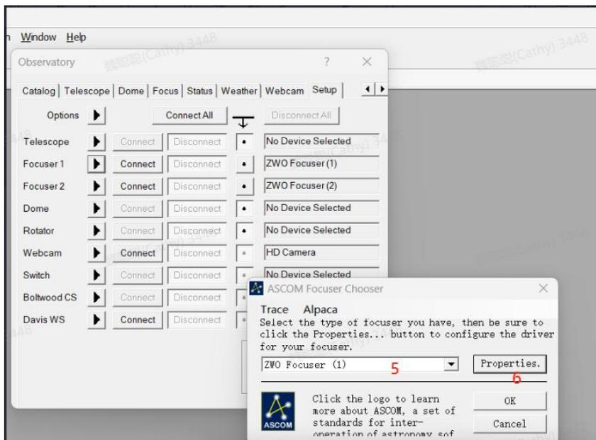
7. Select the USB or Bluetooth connection method, choose the device, and click "Connect" to establish the link. If using EAF Pro for Bluetooth communication, ensure the PC's Bluetooth is turned on, then check the 'BLE' connection option. The system will automatically scan for the device's Bluetooth ID (e.g., EAF Pro\_xxxxxx) and connect to the device.
