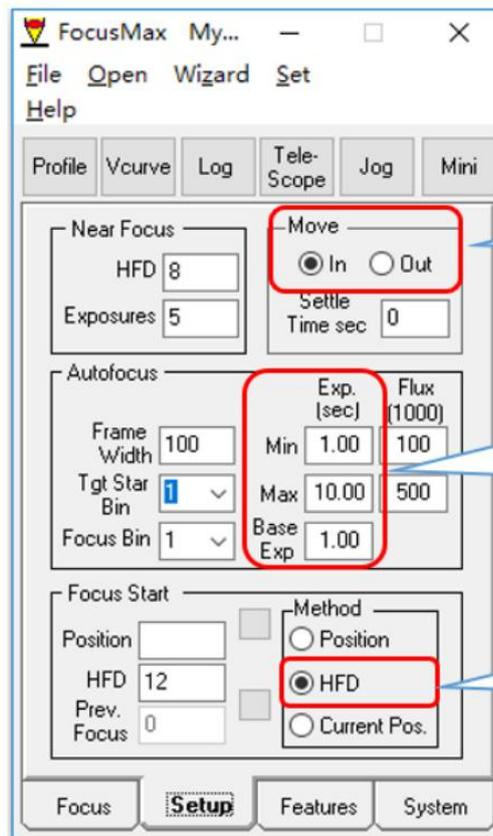
Open the Vcurve dialog box and set the number of steps per move (generally set to -10). Run the autofocus routine.
