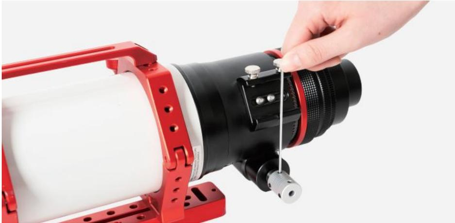
Attach the focuser body to the coupling, align the EAF motor shaft flat surface with the locking screw, and tighten the locking screw using the provided 2mm hex wrench.
