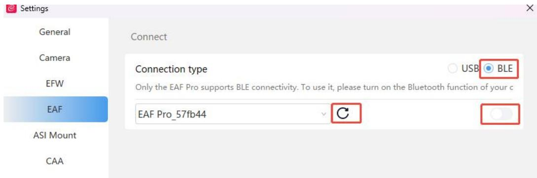
Follow the instructions that pop up on the screen and press the IN or OUT button on the EAF Pro within 60 seconds to pair via Bluetooth. (Once the pairing is successful, the beeping sound from the device will stop.) If Bluetooth was previously connected, re-pairing is not required.
