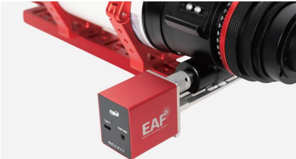
For curved focusers like the one in the image above, you only need to use the original locking screws and 3 washers to secure the EAF. There is a groove at the bottom of the EAF bracket, and a single screw provides sufficient stability.
