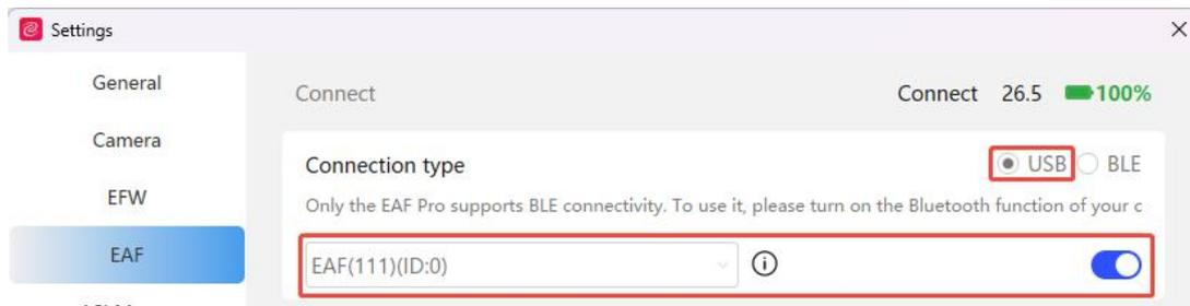
**Bluetooth Communication:** EAF Pro also supports wireless Bluetooth communication (not supported by EAF). First, enable Bluetooth on the PC, then select “BLE” communication method on the “ASISudio”, scan for the Bluetooth device ID, and toggle the connection switch.
