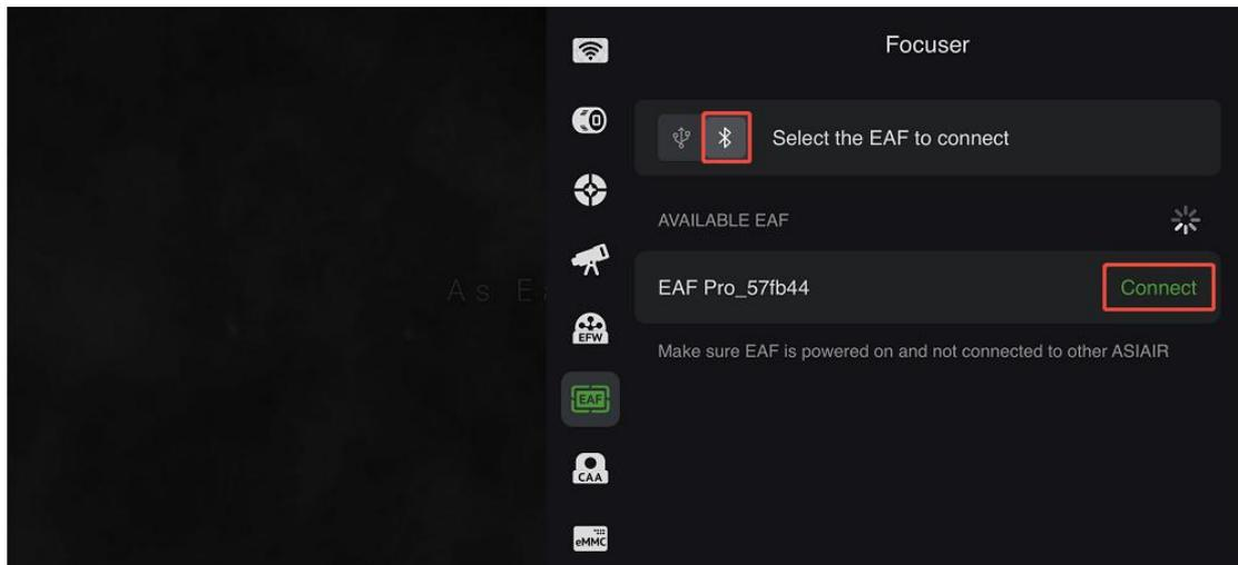
According to the information displayed on the screen, click the IN or OUT button on the EAF Pro body within 60 seconds to pair via Bluetooth (the beeping sound from the device will stop). If Bluetooth has been paired previously, it's no need to repeat the pairing process.
