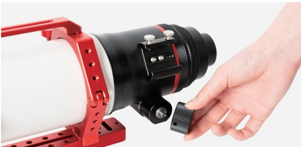
Install the coupling on the telescope focuser shaft and tighten the locking screw with the 2mm hex wrench.
