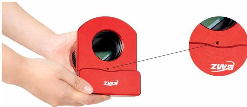
② Then use the standard hexagonal wrench and insert it into the exposed hole;
