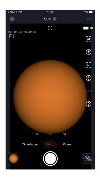
Choose the suitable magnification levels (1x/2x/4x) to observe the Sun, choose the Appropriate field of view, and tap the circular button below to capture a photo.
