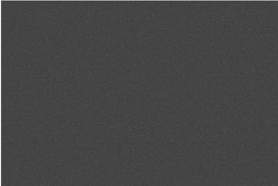
(Dark frame from ASI2600 without any amp glow – 300s exposure time)
